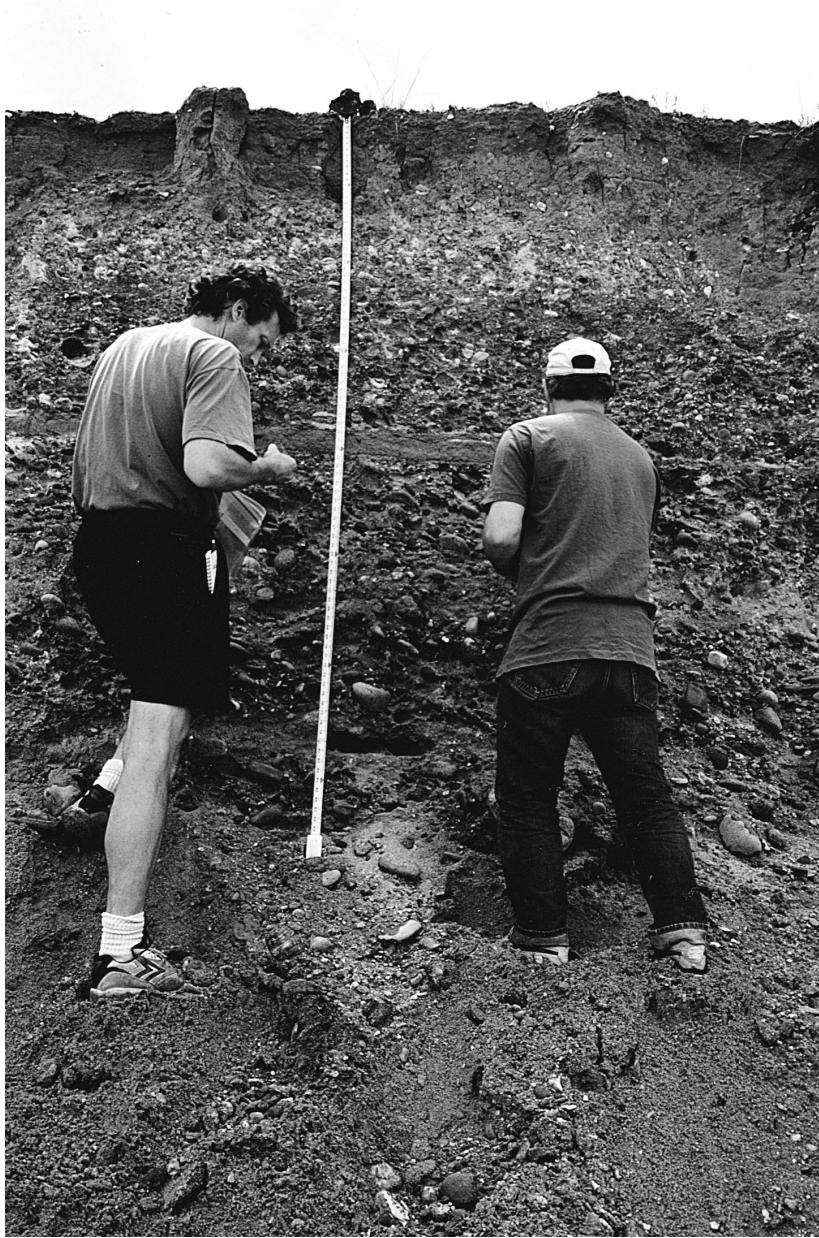
Fig. 5. View of terrace subsurface at sample site 9B showing the imbricated fluvial gravels, thin sand lenses (near middle and bottom of deposit), and capping silt layer (upper \sim 45 cm) that are typical of the deposits of the Wind River terraces. Numerous quartzite clasts (or quartz sands) are collected at several depths in such exposures; equal masses of quartzite are extracted from each clast and combined into one sample. We analyzed samples from several depths to obtain the mean CRN profile in a deposit, which allow an estimation of deposit age and mean inheritance.
